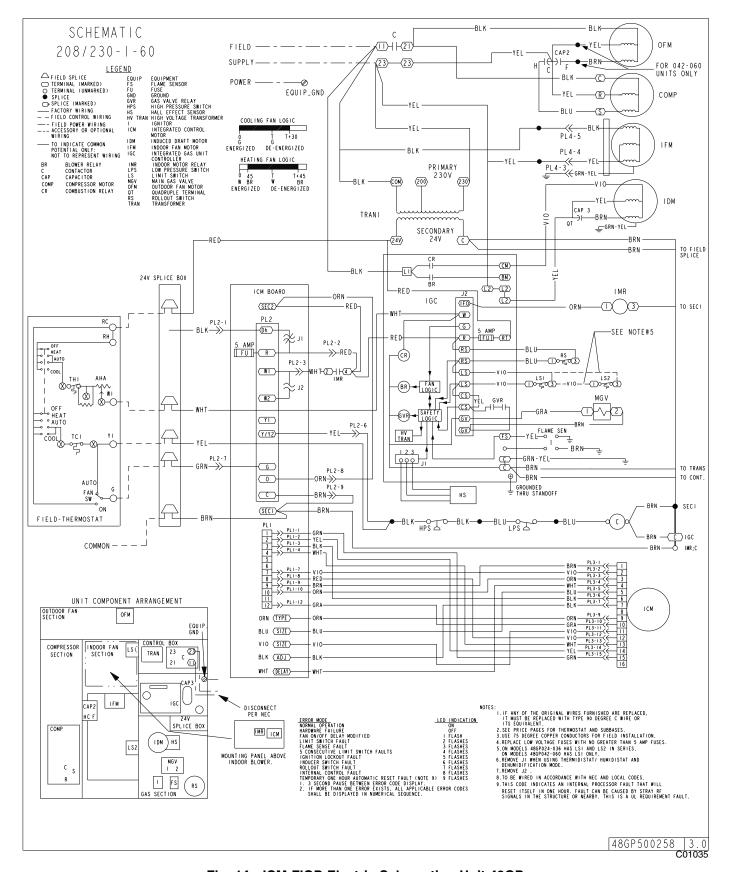
Fig. 14—ICM FIOP Electric Schematic—Unit 48GP
